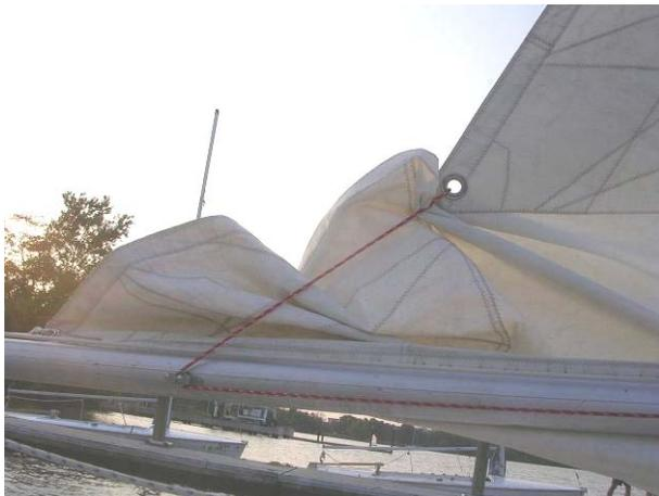
**Step 4:** Pull the red reef line on the boom tight, this will raise the aft end of the boom to the sail while also tightening it. The reef line should be tightened until the sail has a horizontal crease just above the boom. Secure the reef line to the cleat on the forward starboard side of the boom.
