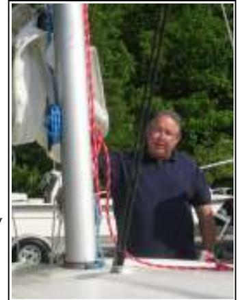
*Photo 3: The line on the starboard side of the mast hoists the main sail; the line on the port side of the mast hoists the jib.*
