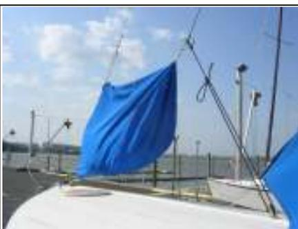
Photo 2: The jib, still hanked onto the forestay, and the jib sheets are stowed in the blue sail bag, which is secured to the pole lift for the spinnaker pole.
