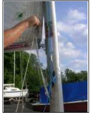
*Photo 5: The Cunningham, which, when tightened, flattens the front of the main sail and allows the skipper to point higher.*
