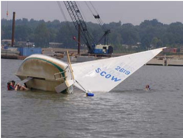
6. Pulling down on the centerboard makes the boat pop up. It may take two people, depending on their weight.
