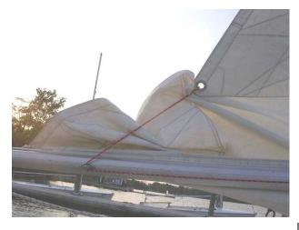
**Step 4:** Pull the red reef line on the boom tight, this will raise the aft end of the boom to the sail while also tightening it. The reef line should be tightened until the sail has a horizontal crease just above the boom. Secure the reef line to the cleat on the forward starboard side of the boom.
