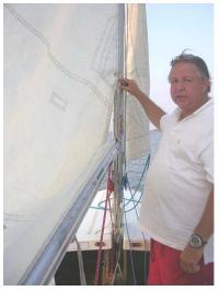
**Step 1:** Lower the main sail to the point where the reef tack cringle (also known as a grommet) is even with the notch in the mast (where one normally inserts the head of the sail when rigging).
