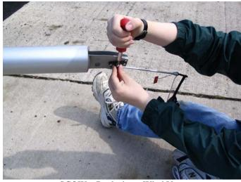
SCOW – Replacing a Wind Vane
