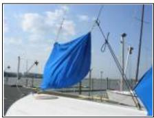
Photo 2: The jib, still hanked onto the forestay, and the jib sheets are stowed in the blue sail bag, which is secured to like buoy balls. the pole lift for the spinnaker pole.
