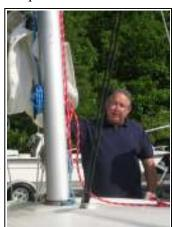
Photo 3: The line on the starboard side of the mast hoists the main sail; the line on the port side of the mast hoists the jib.
