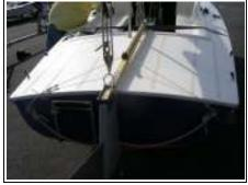
Danschweida also features a tiller tamer to hold the tiller in a fixed position allowing both hands free for other tasks.
