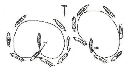
In any COB situation, the first three steps are always the same: Yell, Point, Throw. On a cruiser, if you are under sail, you can use the engine. In very light winds, or in heavy winds, or with an inexperienced crew, the engine may be the best alternative.
